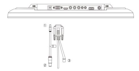
Remind: 1.Please connect port ① to the DC Input of monitor. 2.Please connect port ② and ③ for camera connection.
